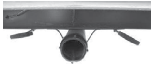
Black/Grey Tank Drain & Valves
