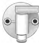
Exterior Fresh Water Drain
