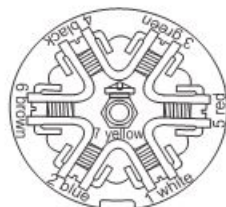
7-Way Trailer Plug- car end rear view
