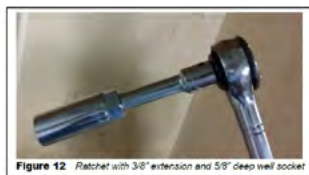
Figure 12 Ratchet with 3/8" extension and 5/8" deep well socket
