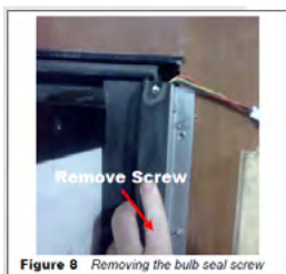
Figure 8 Removing the bulb seal screw
